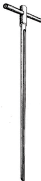
Left: A “dig stick” which can be hammered into soil. Twist and withdraw, then examine soil profile for moisture. Available from Murray Machining, Murray Bridge.
