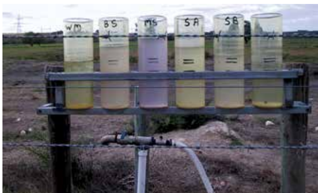
IRRIGAUGES installed and numbered to match watering sections. The black lines mark the irrigation point for summer and autumn/spring.
