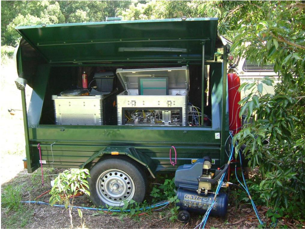
**Figure 4.** Portable automated greenhouse gas sampling unit as used at elected sites within the Nitrous Oxide Research Program in Australia.
