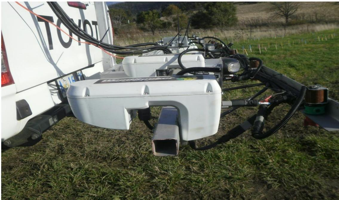
**Plate 1: Smart-N™ WeedSeeker® sensor used in this study.**
